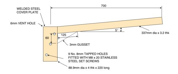
FIGURE 5.1: LIGHTING COLUMN BRACKET
