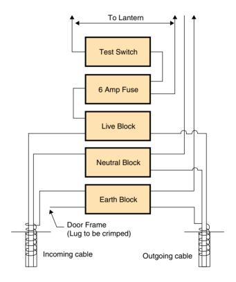
FIGURE 5.2: INTERNAL ELECTRICAL ARRANGEMENT PUBLIC LIGHTING COLUMN
